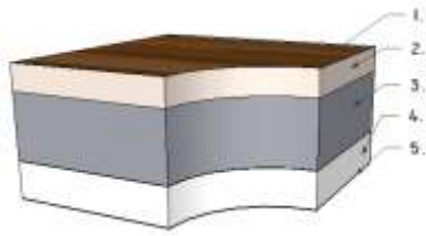
Figure 1: Composition of the ceiling structure before the acoustic measure. 1) wear layer; 2) floor layers with a total thickness 100 [mm]; 3) Reinforced concrete slab thickness of 250 mm (650 [kg/m 2 ]); 4) Polystyrene EPS 140+ light mortar; 5) light mortar with reinforcement mesh+ finish plaster ( m'_2 = 4 [kg/m 2 ], s' = 40 [MN/m 3 ]);
