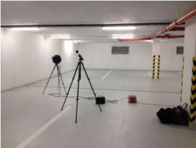
Figure 2: The airborne sound insulation measurement of ceiling structure above the garage.
